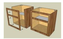
The face frame of the cabinet is typically 1.5" wide and sometimes up to 2" in width. The frame is made of hardwood and is assembled with tongue and groove joints and screws. Doors for framed boxes with either have full overlay or standard overlay. Full overlay will show 1/4" of the frame while standard overlay will show 1" of the frame. Again, your cabinet installer can show you the differences and guide you in your decision.
